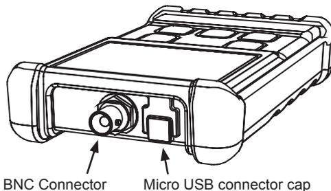
Fig. 15 - Instrument's connectors
