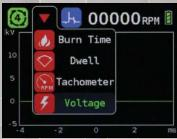
Measures and displays spark burn (firing) time, dwell time, current ramp time, RPM, and spark plug peak voltage.
