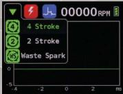
Works on 2-stroke, 4-stroke, and waste spark ignition system engines.
