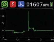
Displays secondary ignition waveforms.
