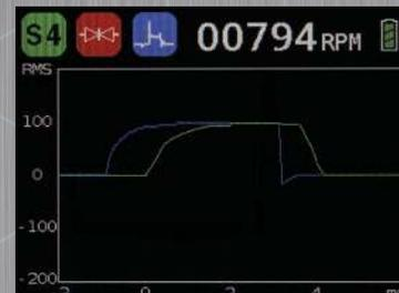
Displays signal voltage, injector power and pintle valve position.
