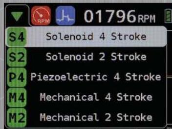
Works on solenoid, piezoelectric and mechanical fuel injectors.
