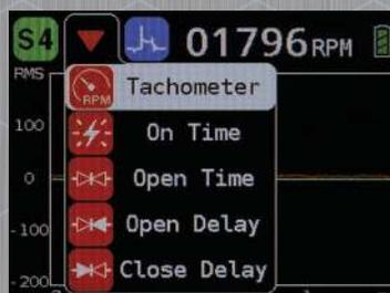
Displays and measures RPM, on time, open time, open delay and close delay.
