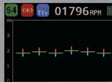
Candle stick graph compares maximum, minimum and average measurements of several injectors.
