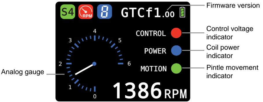
Fig. 8 - Digital display in RPM mode
