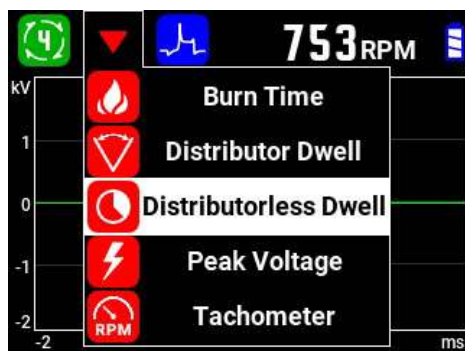
Fig. 6 - Measurement mode selection menu for SPW sensor
